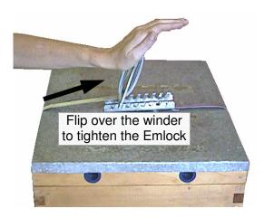
Adjust the strapping tension if necessary. If the Emlock is too loose, unfasten the Emlock and place the winder lugs into the next set of teeth in the base. If the Emlock is too tight, then loosen the winder off by "one set of teeth".
